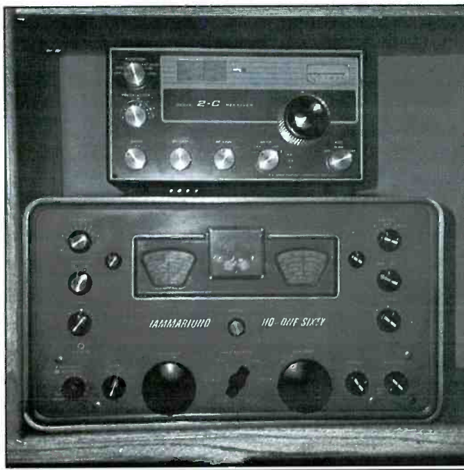
Two trends in receiver development. The larger receiver is the Hammarlund HQ160, while the one on top is the Drake 2C, the successor to the 2B.
