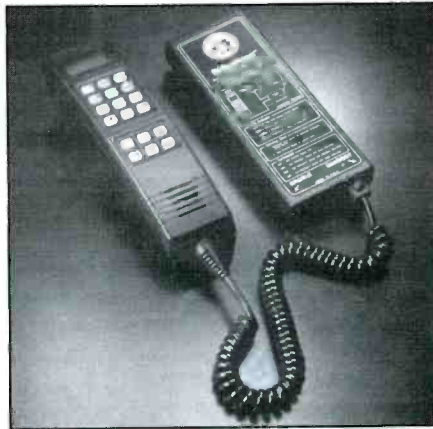
PrivaFone introduced this cellular phone scrambling system that is simple and inexpensive. Photo shows the part of the system that connects to the car-phone.
